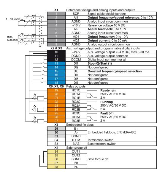
Total load capacity of the auxiliary voltage output +24 V (X2:10) is 6.0 W (250 mA/24 V DC). Wire sizes:
